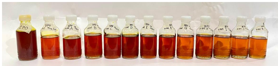
Figure 2. Visual appearance of Crude Palm Oil (CPO) before bleaching and Bleached Palm Oil (BPO) obtained using fresh Bleaching Earth (BE) and Reactivated Spent Bleaching Earth (RSBE A–K). Samples are arranged from left to right as CPO, BE, and RSBE A–K.
