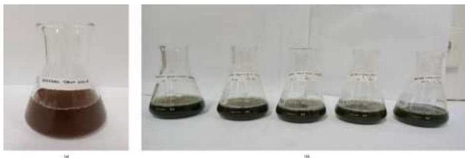
Figure 2. (a) Green betel leaf extract and (b) color change of the extract- Cu(NO_3)_2 \cdot 3H_2O mixtures after 24 h.
