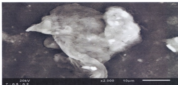
Figure 4. SEM morphology of biodegraded composites with ratio of PP:PP-g-MA: DSS (7:0.5:0.5) before being buried in garbage soil with 2000x magnification
