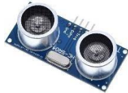
Figure 5. Ultrasonic sensor (HC-SR04)
