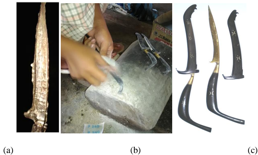
Figure 3. The blades of rencong produced from metal brass waste
