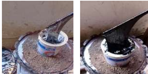
Figure 2 Rubber homogenization process with asphalt
