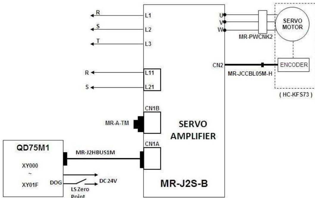
**Figure 2.** Servo Motor Wiring Diagram
