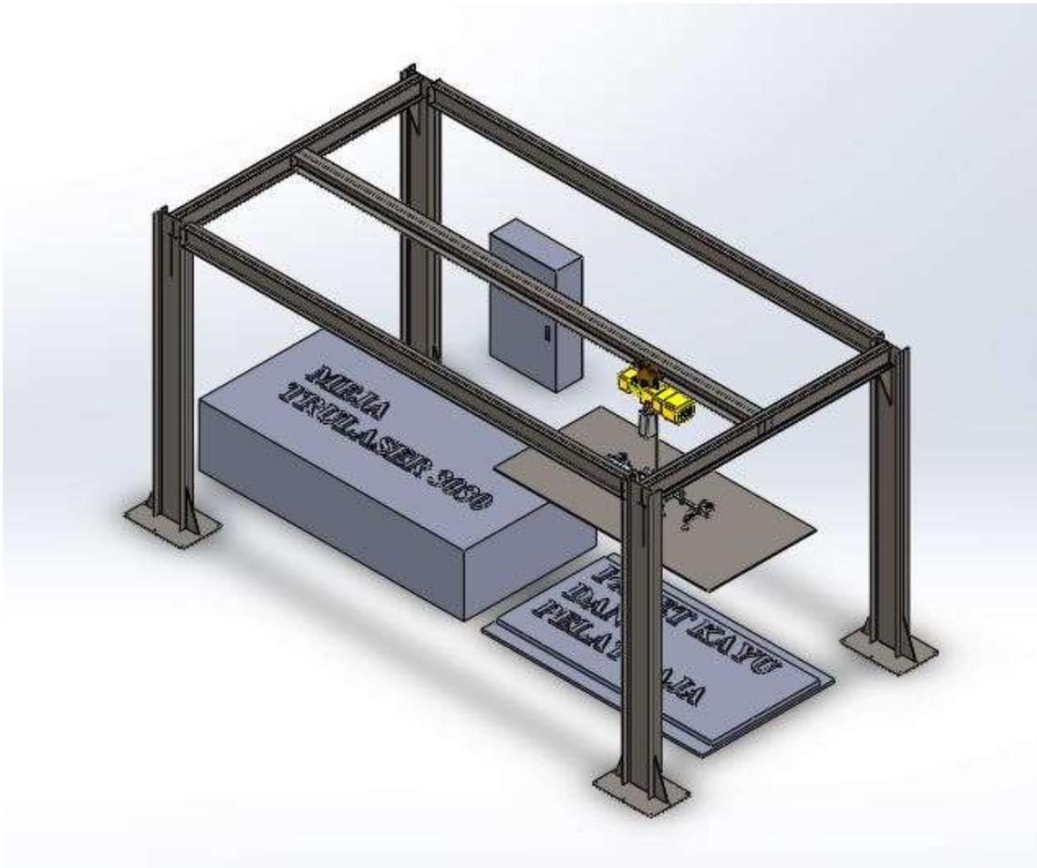
**Figure 3.** Mechanical Design of Steel Plate Transporting Machine (Isometry)
