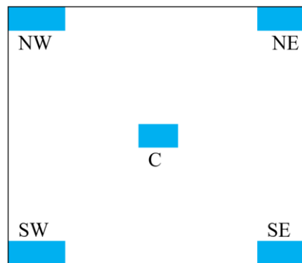
Figure 3. Measuring points for water salinity and pH in the sample plot (Note : NW is Northwest, SW is Southwest, C is Central, NE is Northeast, and SE is Southeast)
