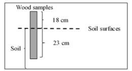
Figure 2. The illustration of graveyard field test
