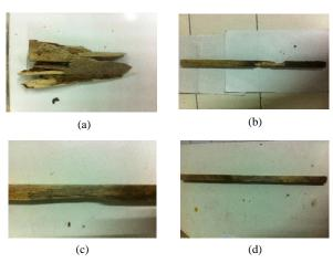
Figure 3. Sengon wood condition after damaged by the subterranean termites (a) untreated wood, (b) 50% ME, (c) MEGSiO<sub>2</sub> 0.5%, and (d) MEGSiO<sub>2</sub> 1%
