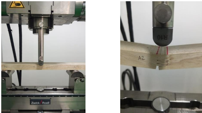
Figure 7. FJL damage during mechanical testing
