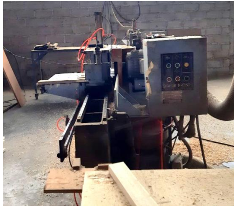
Figure 1. Finger joint machine
