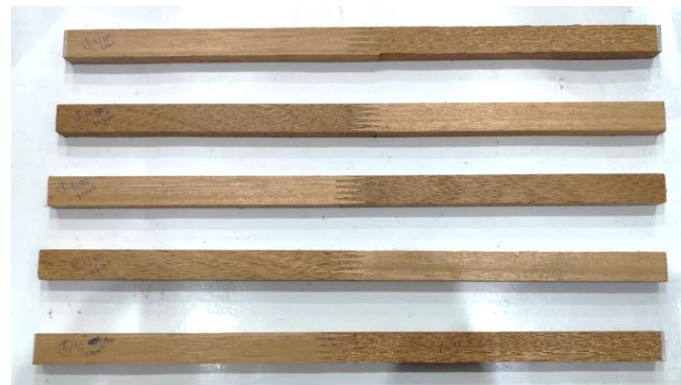
Figure 2. Meranti FJ board samples.
