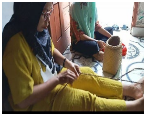
Figure 1. Manual Bulrush String Spinning Process
