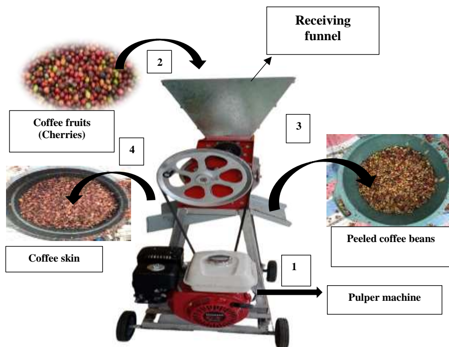
Figure 4. Stages of using a pulper machine
