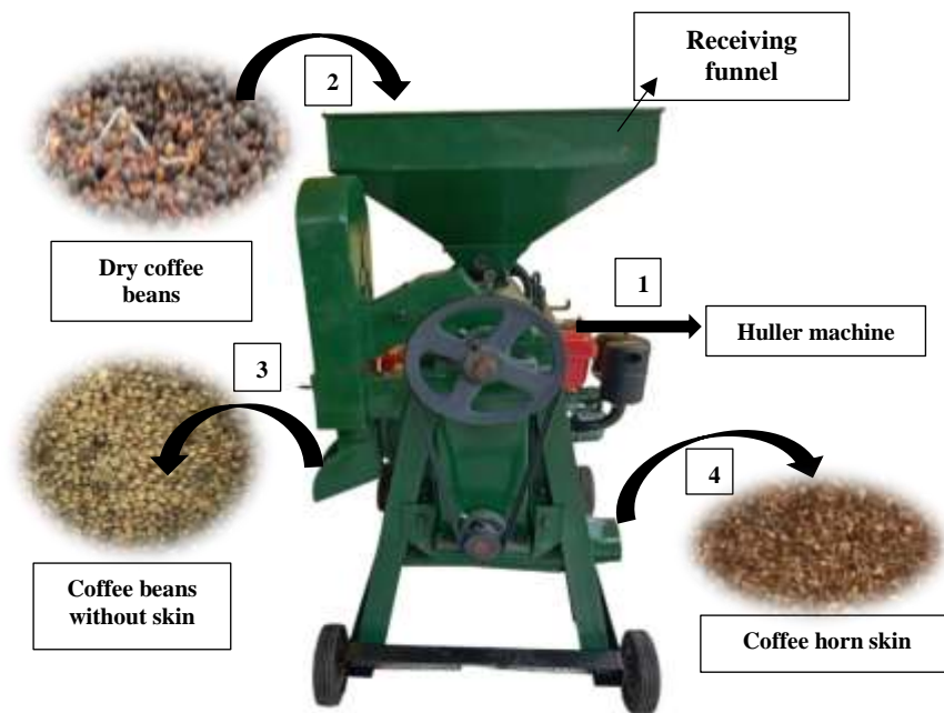
Figure 5. Stages of using a huller machine
