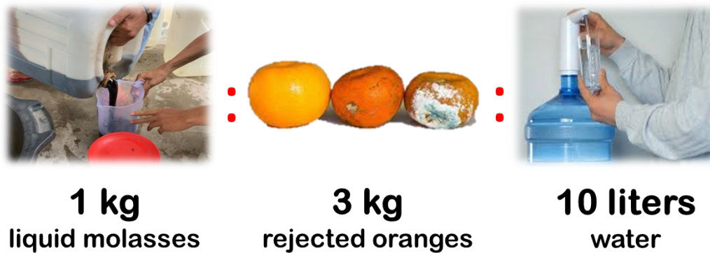
Figure 1. The ratio of materials in the fermentation of rejected oranges
