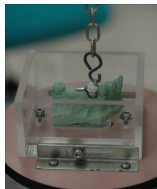
Figure 4. Pulling out the clasp by UTM
