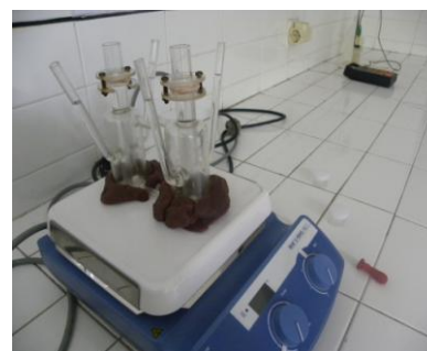
Figure 4. Transport test using Franz Like Difussion Cell
