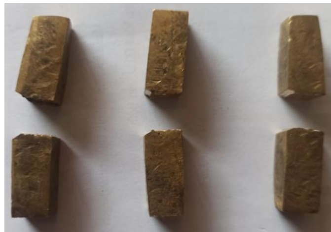
Figure 11. Physical form of fracture of brass material without forging process.
