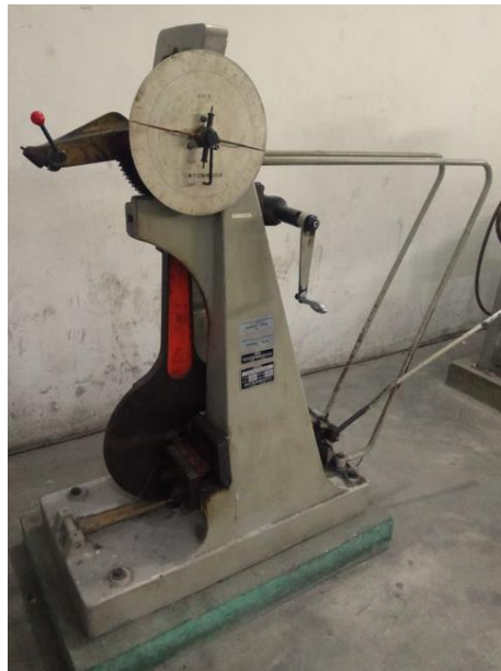
Figure 5. Test tool Charpy Impact Testing Machine type CI-30 TORSEE.
