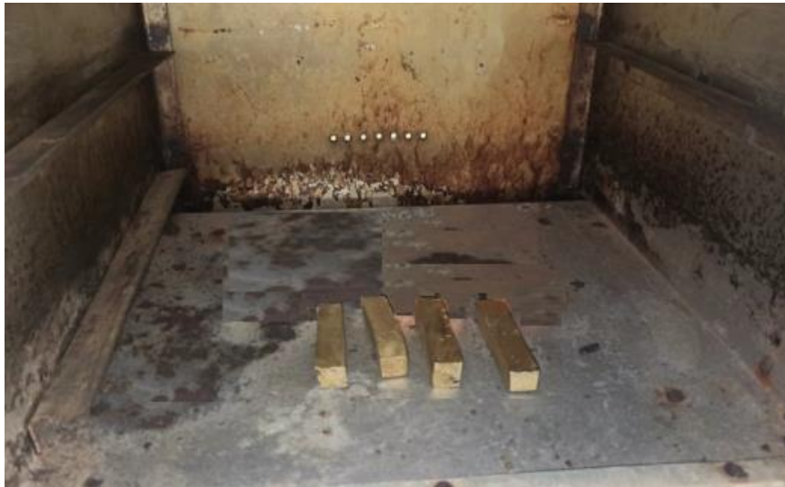
Figure 3. Test specimens for brass material heating process in the oven.
