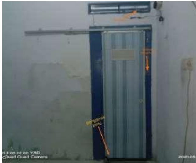
Figure 4. Design of Automatic Sliding Doors with Actuation Mechanics, Ultrasonic Sensors and Arduino Systems.
