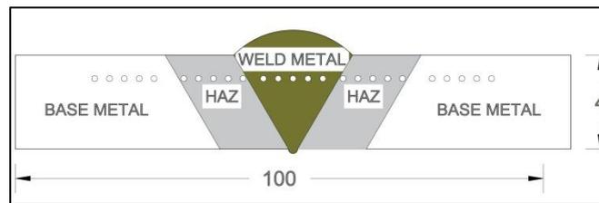
**Figure 3.** Micro-Hardness Test Coupon of AA1135
