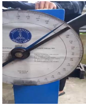
Figure 2.4. Final angular position after testing the specimen.
