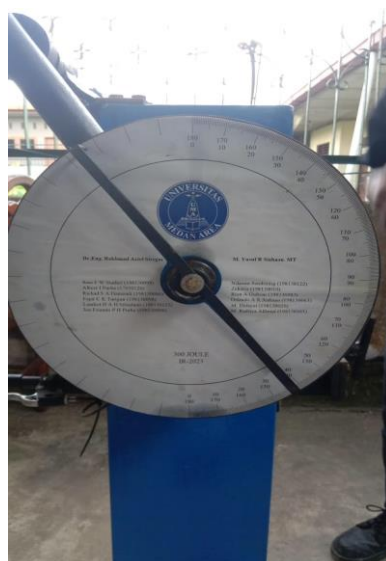
Figure 2.3. Position of the pendulum arm is 147 degrees.
