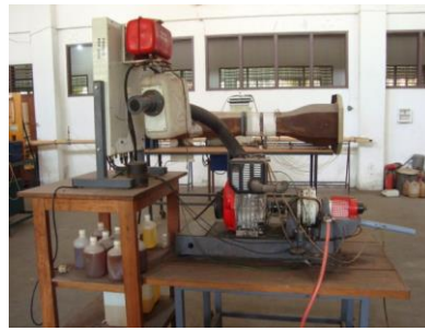
Gambar 3.3 Mesin Uji TD 110 – TD 115 Test Bed and Instrument for Small Engines 4 stroke - 1 cylinder
