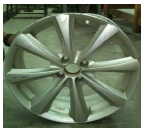
Gambar 1. Velg mobil Toyota Corolla Altis jenis Aluminium Alloy A413.0
