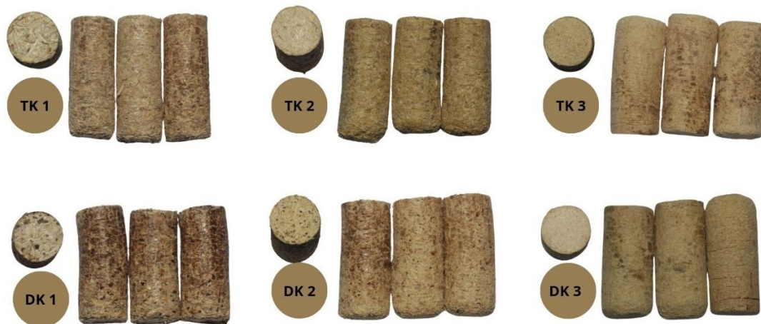
Figure 1. The appearance of calliandra pellets after molding (Notes: TK1 = calliandra without bark with 20 mesh sieve size; TK2 = calliandra without bark with 40 mesh sieve size; TK3 = calliandra without bark with 60 mesh sieve size; DK1 = calliandra with bark with 20 mesh sieve size; DK2 = calliandra with bark with 40 mesh sieve size; DK3 = calliandra with bark with 60 mesh sieve size)
