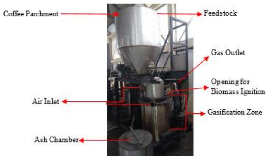
Figure 2. Parts of a downdraft gasifier reactor and the gasification process.
