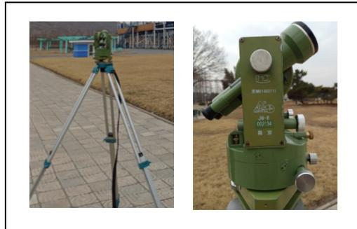
**Figure 2** A Surveyor Installed For The Horizontal Displacement Measurement of The Support Structure
