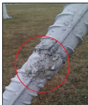
**Figure 4** Butt Weld State of 19mm-Brace
