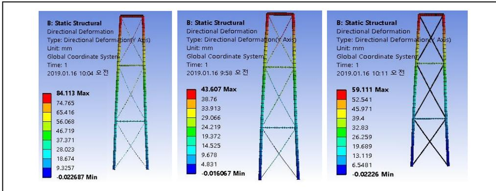
**Figure 14** (c) The Case of The Pre-Stressed Brace (Reinforcing Bar- Φ19mm, Φ32mm, Angle Rolled-Steel Shape 75x5)
