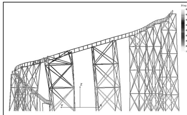
**Figure 17** Analysis Result of Displacement at 5.3602s
