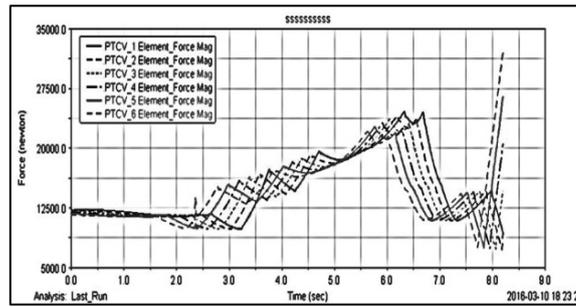
**Figure 16** Load-Time Curve of Each Train of The Roller Coaster Car To The Track
