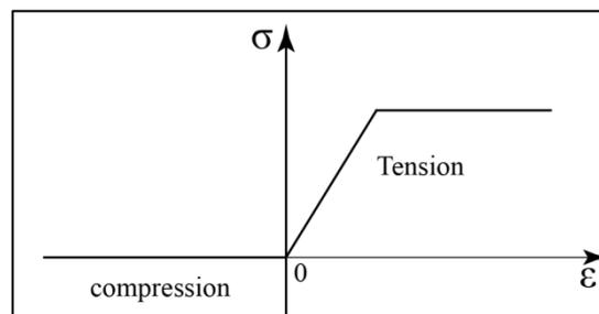
**Figure 11** Nonlinear Elastic Material Model Characteristic Curve
