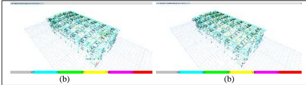
**Figure 8** Evaluation of stress ratio in model 1 at the Tarutung location, SMF system, using methods (a) LRFD, (b) ASD
