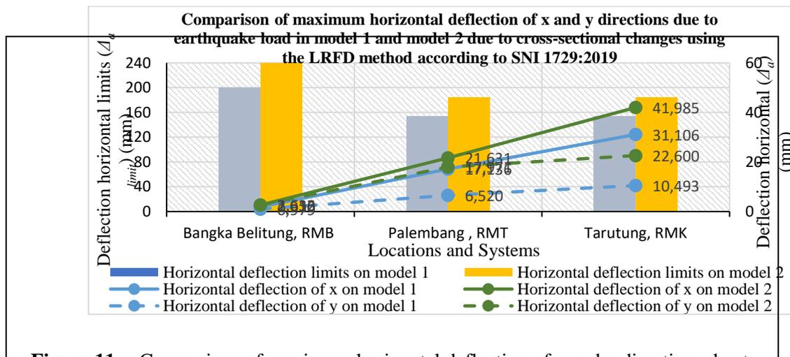
**Figure 11** Comparison of maximum horizontal deflection of x and y directions due to earthquake load in model 1 and model 2 due to cross-sectional changes using the LRFD method according to SNI 1729:2019
