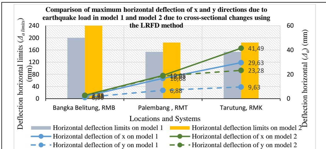
**Figure 12** Comparison of maximum horizontal deflection of x and y directions due to earthquake load in model 1 and model 2 due to cross-sectional changes using the LRFD method according to SNI 1729:2019
