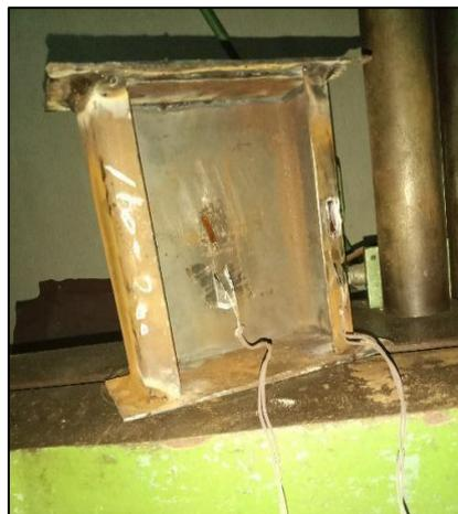
**Figure 6** Member with strain measuring device
