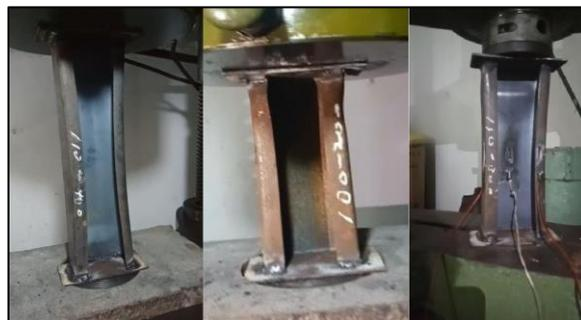
**Figure 7** Members broken by buckling loss
