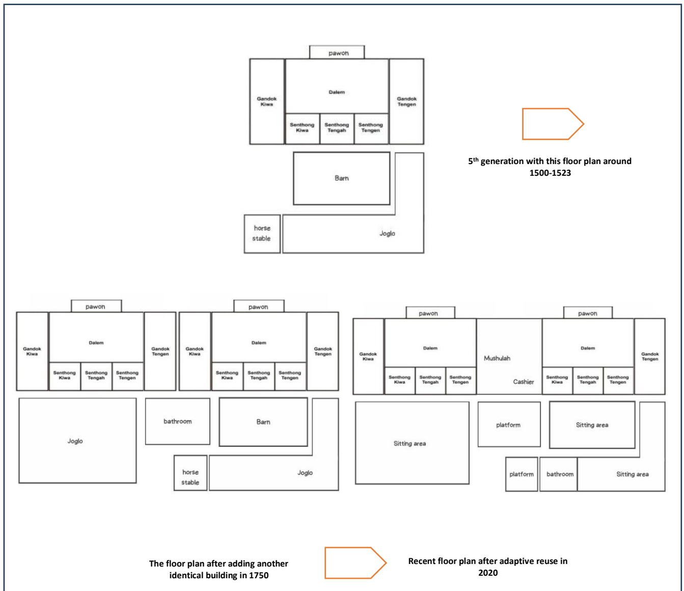
Figure 13 Floor plan BEFORE and AFTER adaptive reuse
