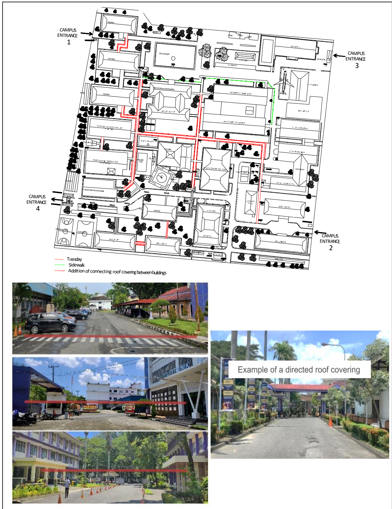
Figure 8 Directional plan for adding a roof covering and increasing the width of the sidewalk
