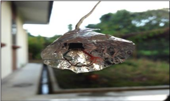
Figure 4 A thermocouple wrapped with the aluminum foil to minimize solar radiation
