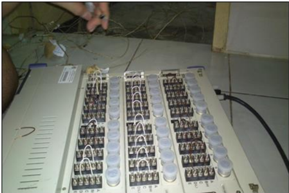
Figure 5 Thermocouples connected to the data logger
