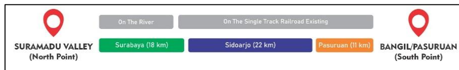
Figure 4. Typology diagram and division of MRT line distance in Surabaya without land acquisition by utilizing the river routes and the existing single track railroad
