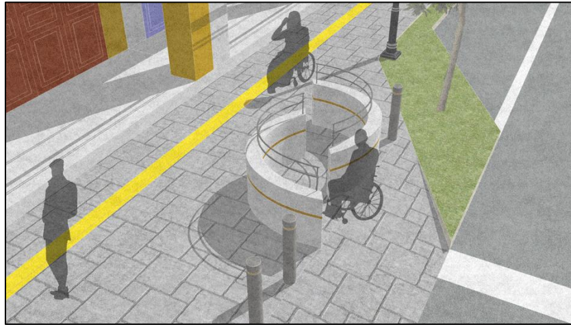
Figure 19. Ramp and S portal barrier
