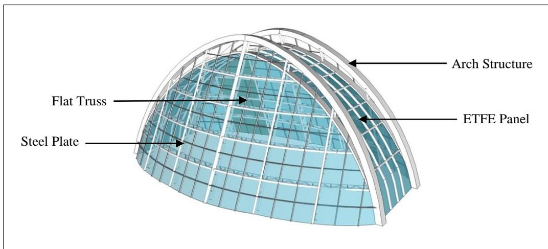
**Figure 4.** Application of Exposed Frame and ETFE Panel
