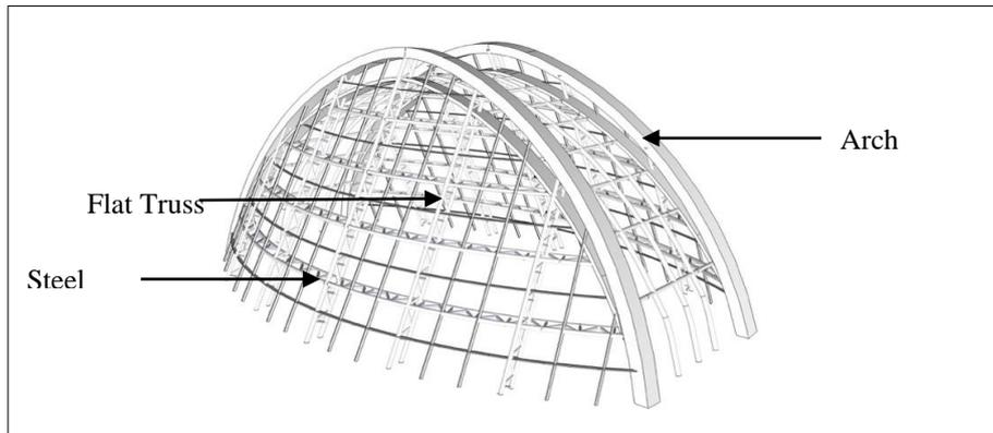
Figure 12. Structure System Concept
