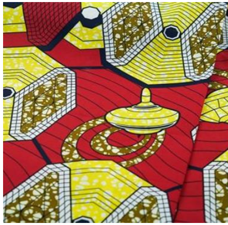
Figure 7. Imitation African Prints: These textiles are produced through direct roller printing techniques, which replicate the characteristic white spots and cracked lines found in African wax prints.
