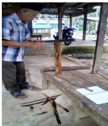
Figure 16. Slitting of Trep Wood slats
