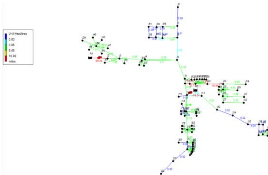
Figure 11. Unit headloss distribution map predicted at all pipes.
