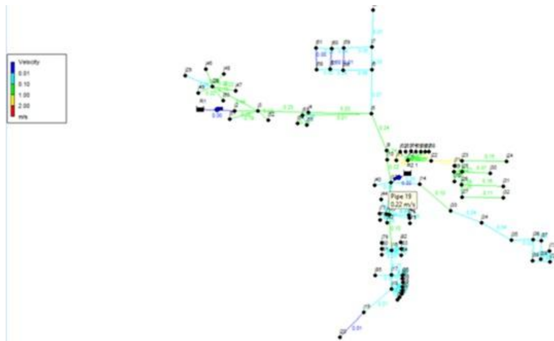
Figure 10. Velocity distribution map predicted at all pipes.
