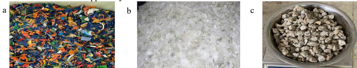
Figure 1 (a) HDPE plastic waste pieces; (b) PET plastic waste; (c) pumice.
