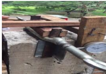
Figure 5. How to install Dial Indicator and Turtle
