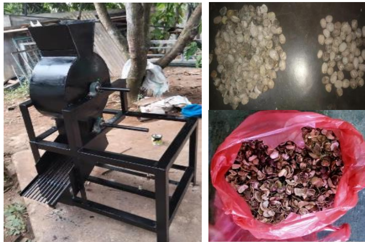
Figure 2. a) Built in overall machine design; b) seed flesh and cracked shell
