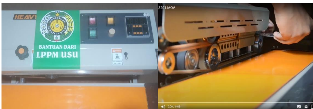
Figure 6. Continuous band sealer semi-automatic machine.
