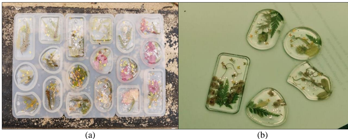
Figure 4 (a) Resin key chain in the drying process, (b) Resin key chain product that has been dried and removed from the mold.
