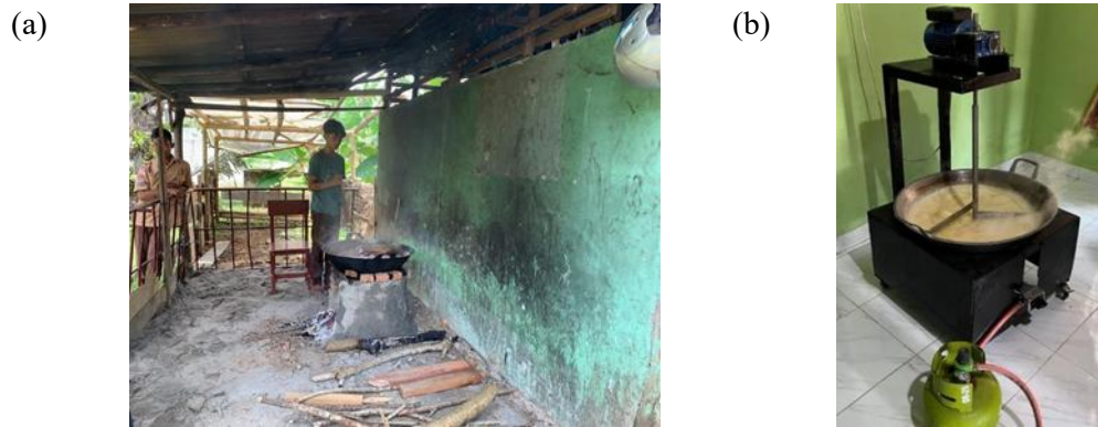
Figure 7. (a) Traditional firewood-based cooking of palm sap, (b) modern cooking technology introduced during the community service program.
