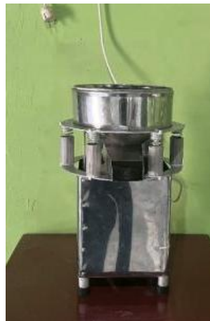
Figure 6. Palm sugar sieving machine.
