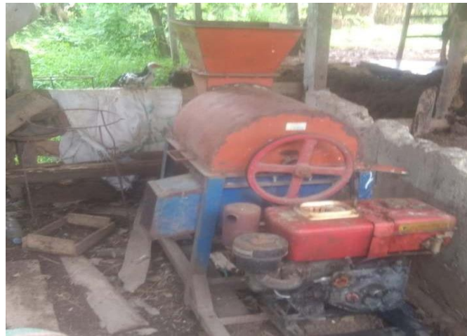
Figure 5. Chopper machine for chopping grass and organic fertilizer for Alebo Village Farmers Group
