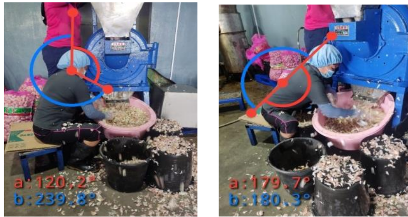
Figure 4. RULA measurement position B; (a) neck, (b) trunk and leg.
