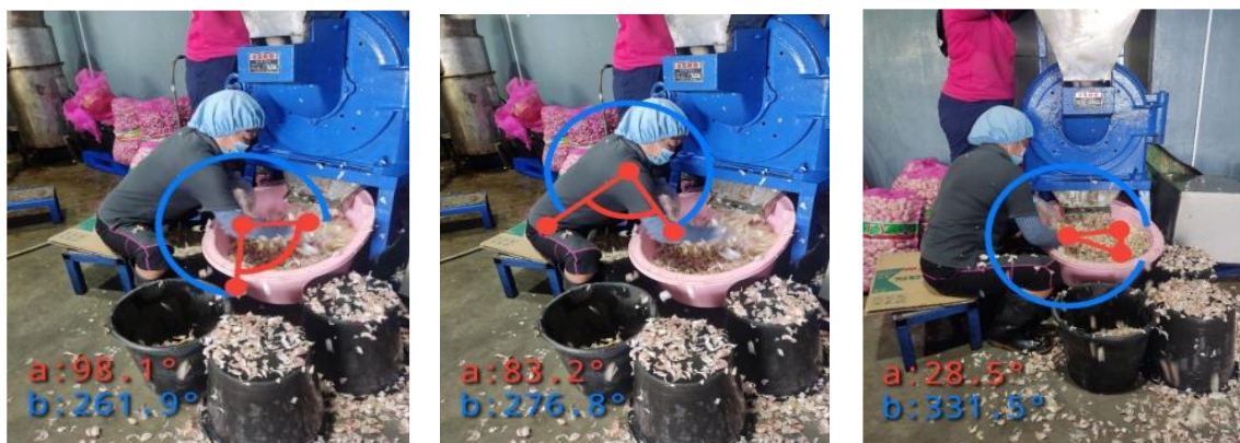
Figure 3. RULA measurement position A; (a) upper arm; (b) lower arm; (c) wrist.
