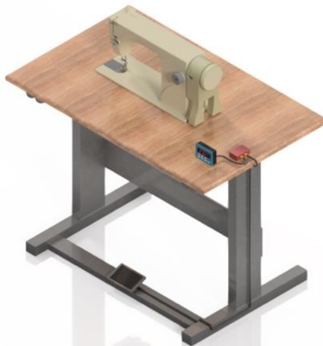
Figure 8 Alarm Timer Integrated into Sewing Machine
