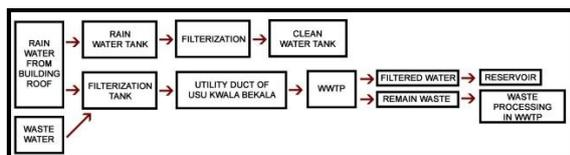
**Figure 20.** Wastewater Scheme with Water Treatment System
