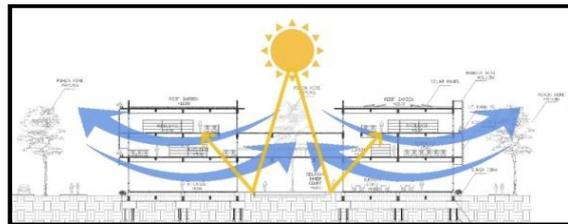
**Figure 14.** Inner Court Scheme which Explains the Movement of Natural Air and Lighting
