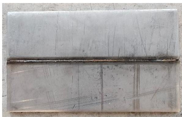
Figure 11. Top view of distortion result in butt joint experiment
